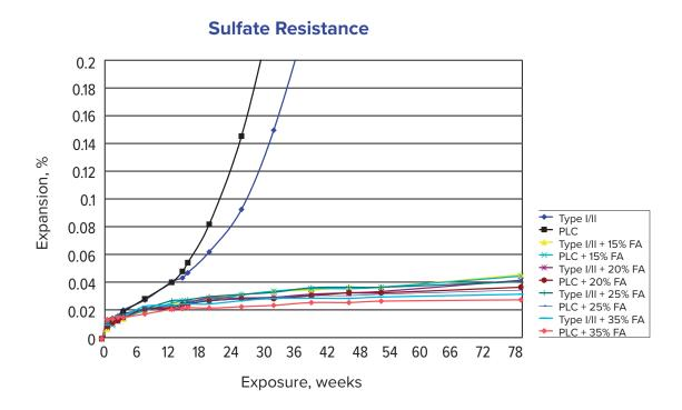
ASTM C1012 **Sulfate Resistance** testing with a wide range of portland cements and portland-limestone cements, with or without fly ash, shows the limestone addition has no impact.
