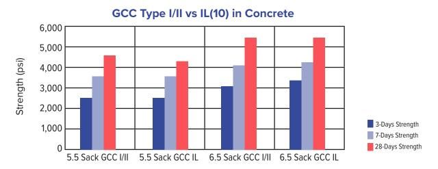
Early and late **concrete strengths** are similar in PLC and OPC. These tests have water/cement ratio of 0.49 for the 5.5 sack mix and water/cement ratio of 0.40 for the 6.5 sack mix.
