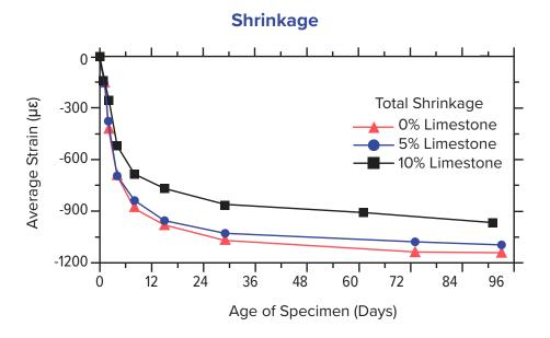
**Total shrinkage** is the autogenous shrinkage plus the free (drying) shrinkage. Shrinkage is measurably lower at 10% limestone. (ASTM C157)
